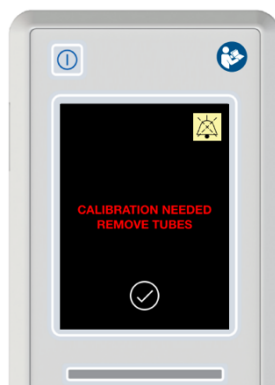
Figure 7: TrachFlush detects tubes are not disconnected
